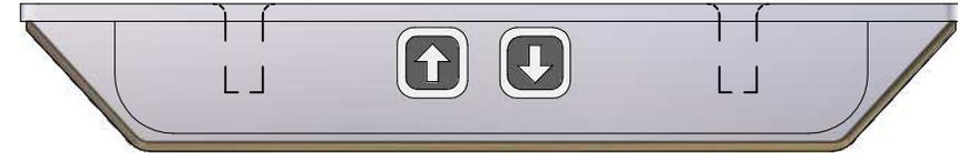
**Initialization of the DL4 parallel systems** (only necessary if legs lose their positions-this is recognized by the TV being able to lower but not raise again)
