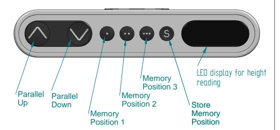
Initialization of the parallel systems (only necessary if legs lose their positions-this is recognized by the desk being able to lower but not raise again)
