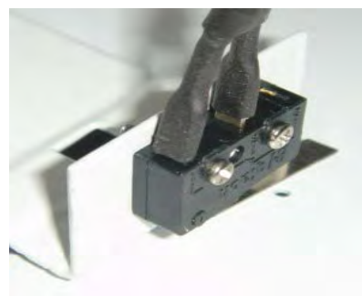
Additional microswitch to lower lift if remote control does not work (Insert pin into hole of ceiling plate to activate switch and lower the lift)
