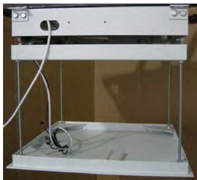
Assembly of the additional IR eye and microswitch in to the ceiling plate
